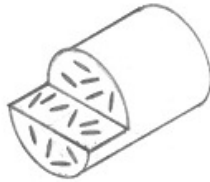
Short fiber thermoplastic material, granules with fiber length up to 1 mm
